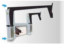
Place the LARGE Bracket in the superior LEFT hook of the plate (from viewer's position), and secure the spring on the bottom hook of the plate.
